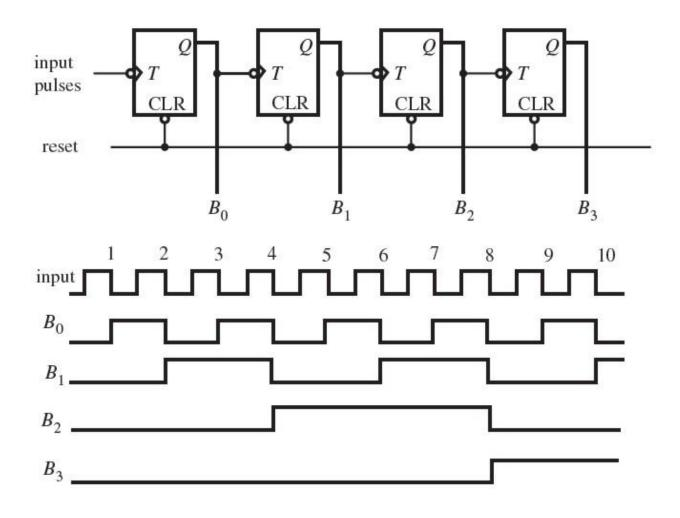
library ieee; use ieee.std\_logic\_1164.all; use ieee.std\_logic\_unsigned.all; entity vhdl\_binary\_counter is port(C, CLR : in std\_logic; Q : out std\_logic\_vector(3 downto 0)); end vhdl\_binary\_counter; architecture bhv of vhdl\_binary\_counter is signal tmp: std logic vector(3 downto 0); begin process (C, CLR) begin if (CLR='1') then tmp <= "0000"; elsif (C'event and C='1') then  $tmp \leq tmp + 1;$
