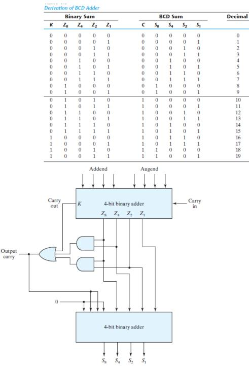
✤ A BCD adder that adds two BCD digits and produces a sum digit in BCD is shown in Fig. The two decimal digits, together with the input carry, are first added in the top four-bit adder to produce the binary sum.
