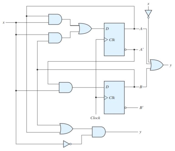
Fig: Example of sequential circuit
