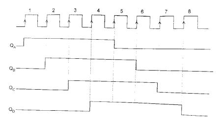
Fig. : Timing Diagram of Johnson Counter
