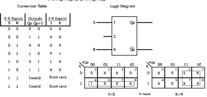
J-K Flip Flop to S-R Flip Flop
