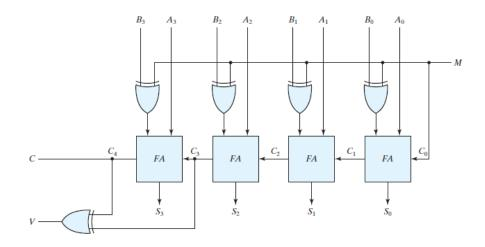
The mode input *M* controls the operation. When M = 0, the circuit is an adder, and when M = 1, the circuit becomes a subtractor.
