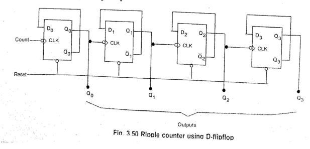
module ripple\_counter  $(Q_3, Q_2, Q_1, Q_0, count, reset);$
