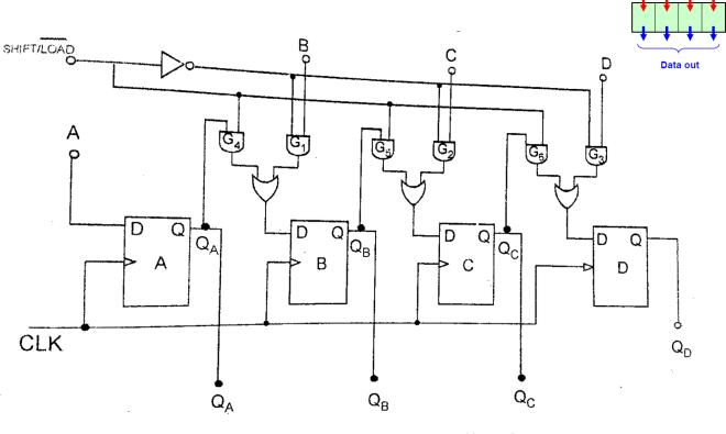
Fig. : Parallel in parallel out shift register
