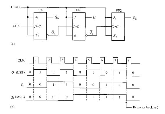
Asynchronous counters are commonly referred to as ripple counters for the following reason: The effect of the input clock pulse is first "felt" byFFO. This effect cannot get to FF1 immediately because of thepropagation delay through FF0. Then there is the propagation delaythrough FF1 before FF2 can be triggered. Thus, the effect of an inputclock pulse "ripples" through the counter, taking some time, due topropagation delays, to reach the last flip-flop.
