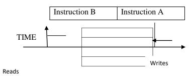
• This is quite common and called **read after write data hazard.** This situation is solved with a simple hardware technique called **operand forwarding.**
