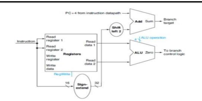
The datapath for a branch uses the ALU to evaluate the branch condition and a separate adder to compute the branch target as the sum of the incremented PC and the sign-extended, lower 16 bits of the instruction (the branch displacement), shifted left 2 bits.
