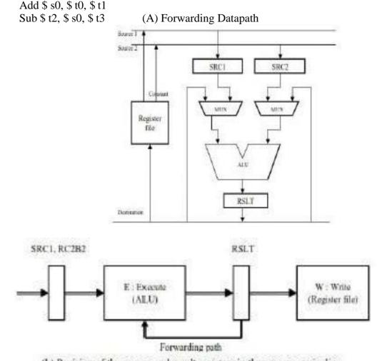
(b) Posision of the source and result registers in the processor pipeline.
