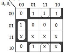
$E_2 = B_2 B_1' B_0' + B_2' (B_0 + B_1)$ For E<sub>0</sub>
