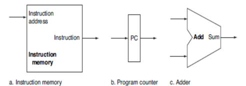
Two state elements are needed to store and access instructions, and an adder is needed to compute the next instruction address.
