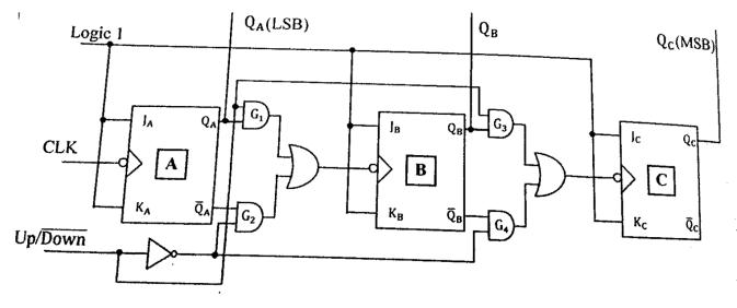
Figure3-bit asynchronous up/down-counter
