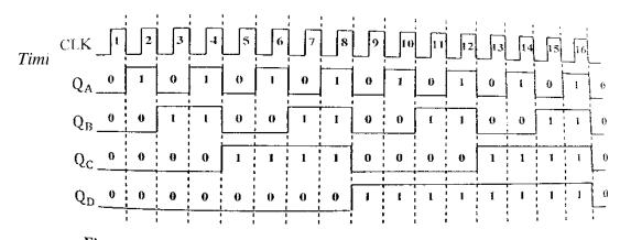
Figure 4.37 Timing diagram of 4-bit asynchronous up-counter.
