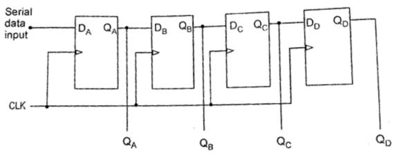
Fig. 3.42: Serial in parallel out shift register
