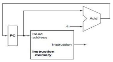
A portion of the datapath used for fetching instructions and incrementing the program counter. The fetched instruction is used by other parts of the datapath.
