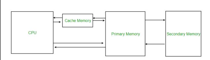
**Cache Memory** is a special very high-speed memory. It is used to speed up and synchronizing with high-speed CPU. Cache memory is costlier than main memory or disk memory but economical than CPU registers. Cache memory is an extremely fast memory type that acts as a buffer between RAM and the CPU. It holds frequently requested data and instructions so that they are immediately available to the CPU when needed.
